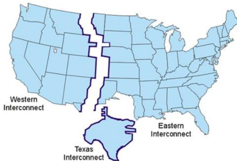
Figure 6-8 North America electric power grids [140]
