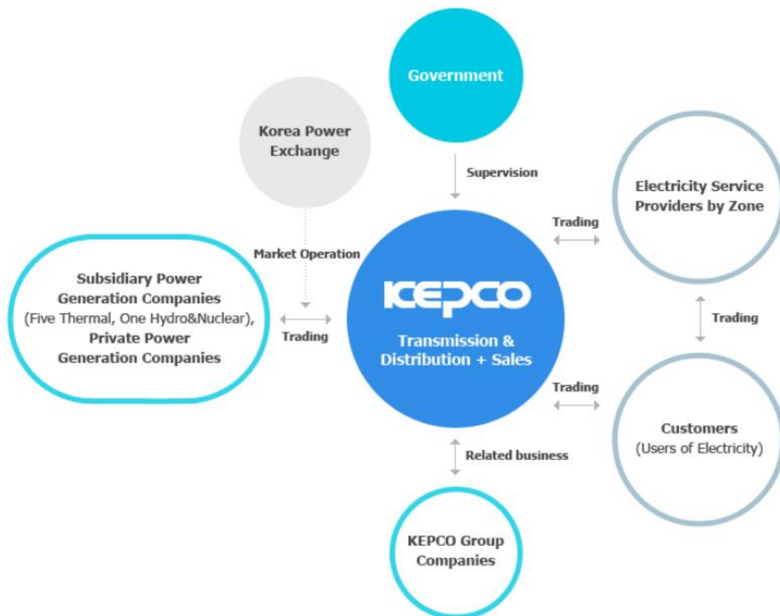
Figure 4-16 Structure of Korea's electric power industry [87]
