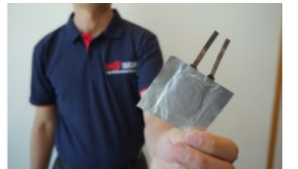
Thermo-electrochemical capacitor device/Conversion of low-grade waste heat into electricity
