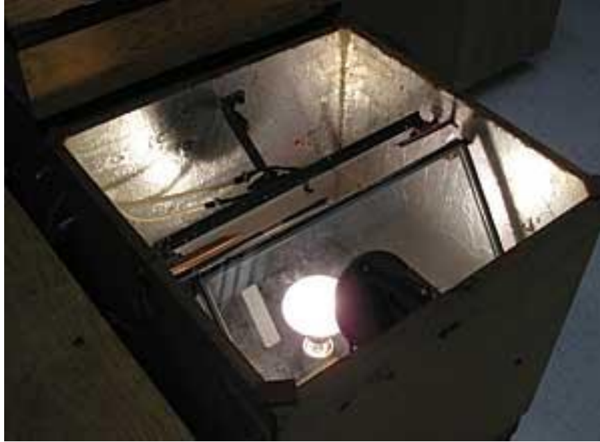
Fog-box used for out-gas testing an insulating glass unit.
