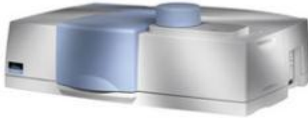
Integrating sphere spectrophotometer.
