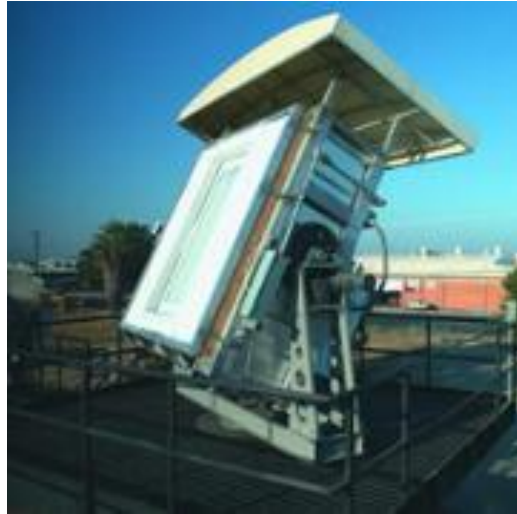
Custom-made solar calorimeter for testing windows.
