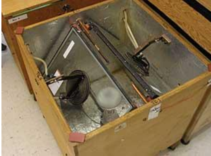
Testing apparatus for testing Argon or Krypton gas fill of insulating glass units.
