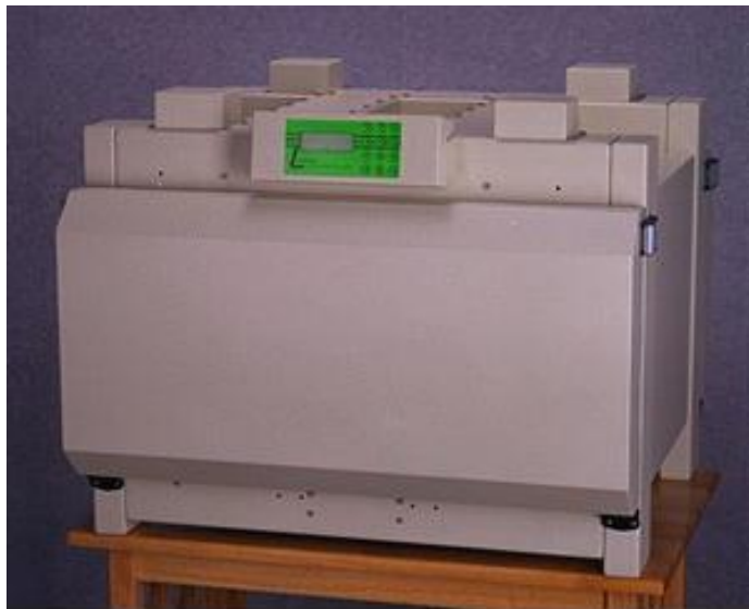
Typical heat flow meter testing apparatus.
