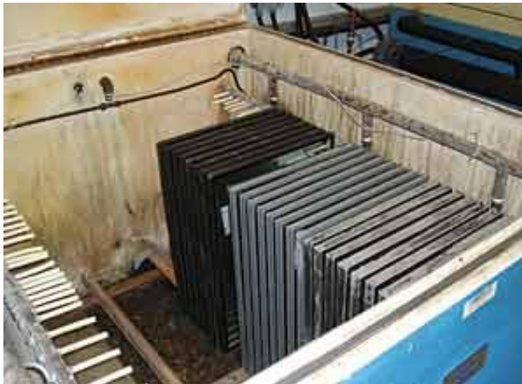
Testing apparatus for humidity and temperature testing of insulating glass units.
